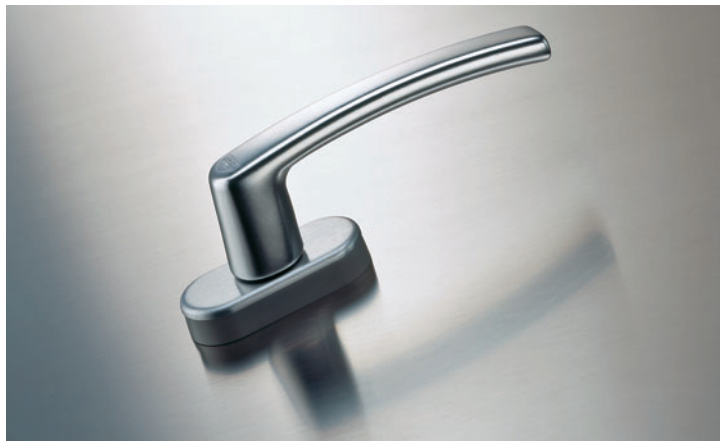
RotoLine Secustik® window handle, 45° click, 32mm spindle length, with Ø10mm lugs – with Roto logo
