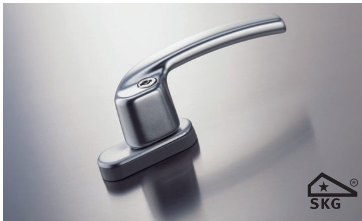
RotoLine cranked handle, lockable – keyed-alike locking, push cylinder – 43mm spindle length, with Ø10mm lugs, 24mm escutcheon cover, including 1 nickel-plated turn-key – without Roto logo, with SKG* logo
