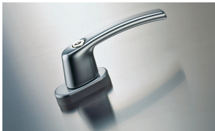
RotoLine window handle, 40Nm lockable, keyed-alike (K.A.) locking, rotary cylinder 35mm spindle length, with Ø10mm lugs, including 1 nickel-plated turn-key – without Roto logo
